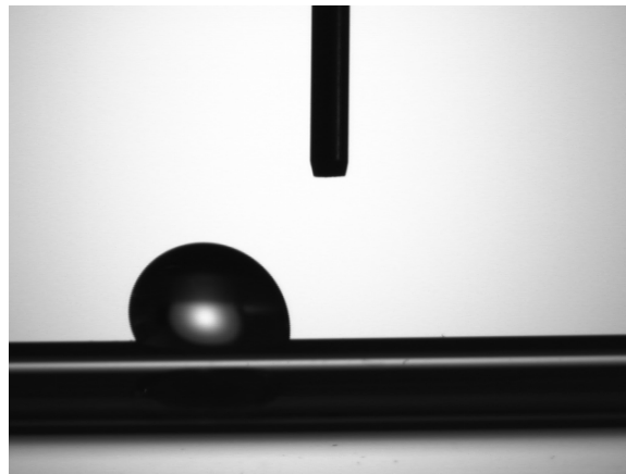
Figure 1. Captured image of a droplet undergoing sliding during intermittent rotation used for sliding angle analysis of an extruded plastic tube.
