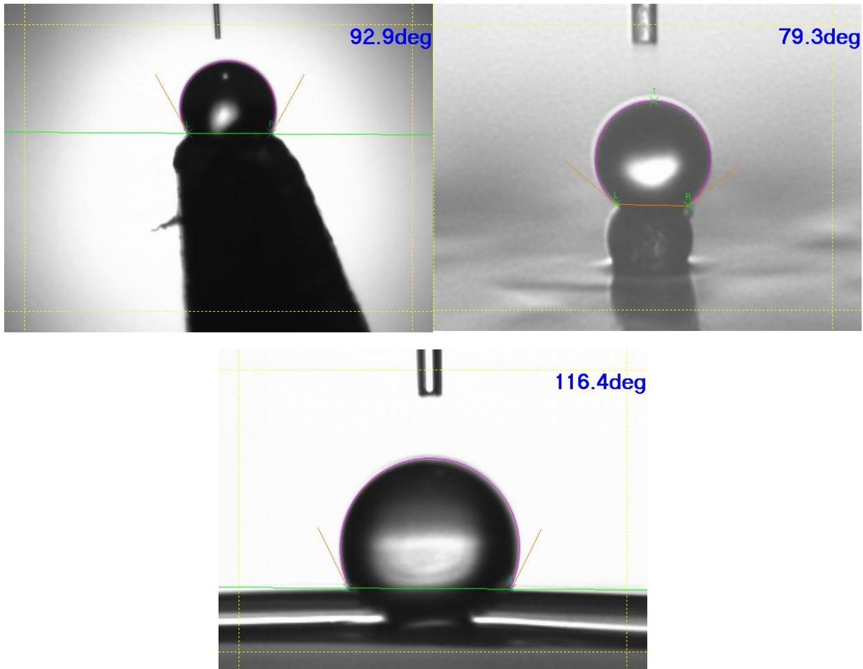
Figure 1. Captured droplets used for micro contact angle analysis on a 140  $\mu\text{m}$  hydroxyapatite coated Ti post (top left), 30 $\mu\text{m}$   $\text{Al}_2\text{O}_3$  particle (top right) and 20 $\mu\text{m}$  polymer fiber (bottom).
