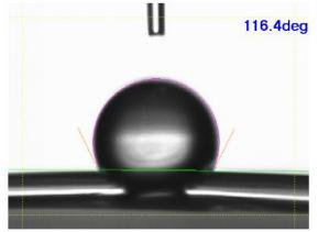
Captured droplets used for microcontact angle analysis on a 140 µm hydroxyapatite coated Ti post (top left), a 30 µm Al<sub>2</sub>O<sub>3</sub> particle (top right) and a 20 µm polymer fiber (bottom).
