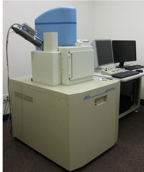
The JEOL JSM-6610LV SEM with Bruker QUANTAX 200 EDS system.
