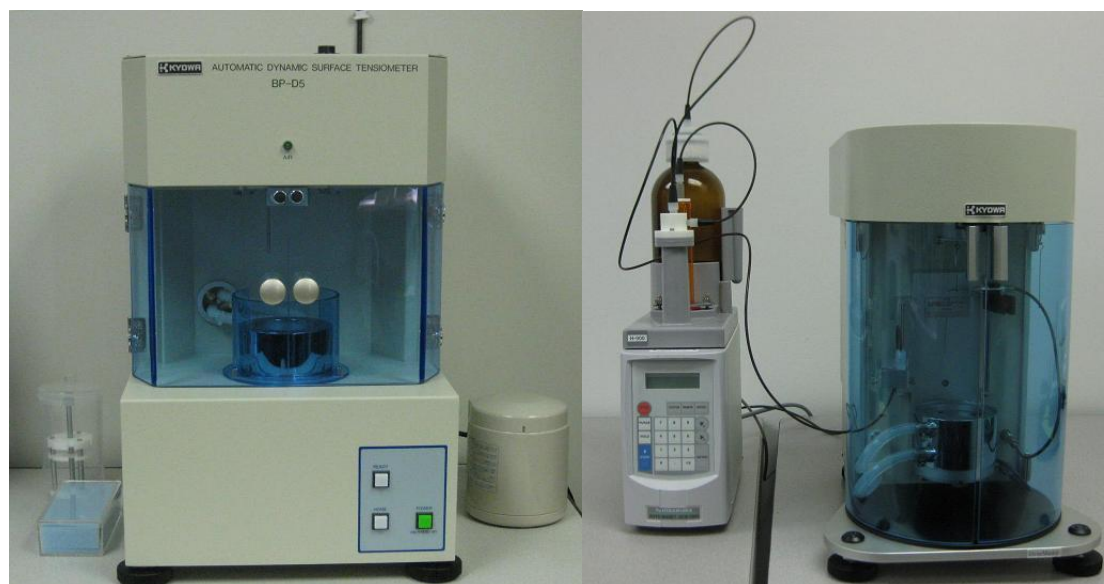
Kyowa BP-D5 (left) and Automatic CMC Measurement Option with a DY-700 Tensiometer (right)
