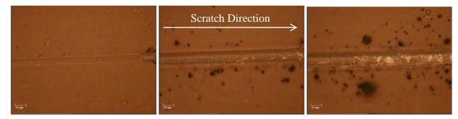
Optical micrographs of the scratch track showing the failure characteristics of the DLC coating on M2 steel; the centers of the scratch track images corresponding to  $L_{c 1}$  (left image, cohesive cracking),  $L_{c 2}$  (center image, adhesive spallation),  $L_{c 3}$  (right image, gross adhesive spallation).
