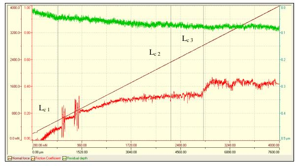
Scratch test data for a DLC coating on M2 steel; the vertical grey lines mark the critical failure points and the corresponding normal forces are critical loads: L<sub>c 1</sub>, L<sub>c 2</sub> and L<sub>c 3</sub>.
