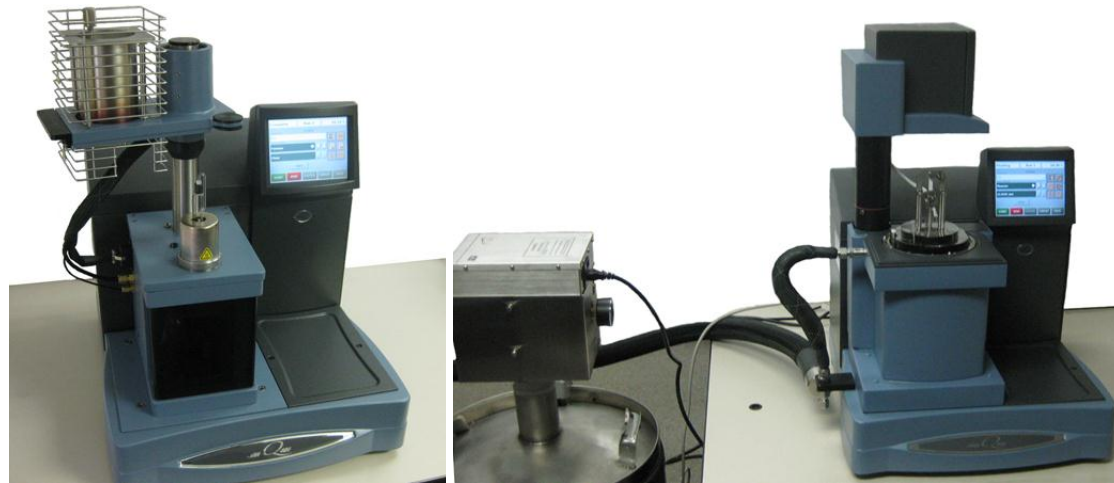
TA Instruments Q400 TMA (left) and Q800 DMA with Gas Cooling Accessory (right)
