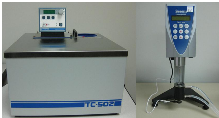
Brookfield Engineering TC-502D Circulator Bath (left) and DV-II+Pro Viscometer (right)
