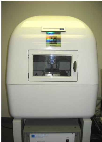
The full-feature, multi-technique nanoindenter; Left: main unit; Right: transducers mounted on a granite platform inside the environmental enclosure.
