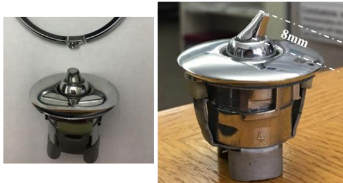
Figure 1. Images of hood ornament after fracture.
