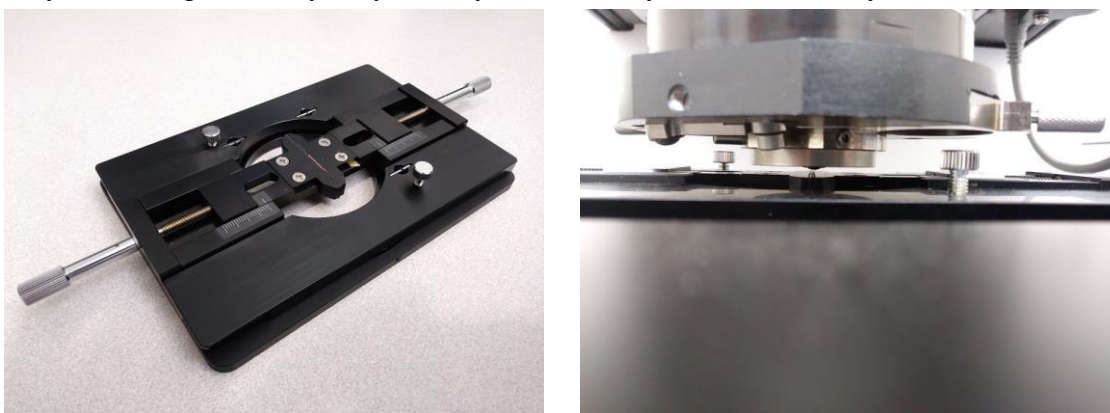
Figure 1. The microvice holder (left) containing a small red sample that has been cross-sectioned and the microvice holder under the germanium ATR microscope accessory (right). (Note: A red sample was chosen for illustrative purposes. It was not the sample that was analyzed.)
