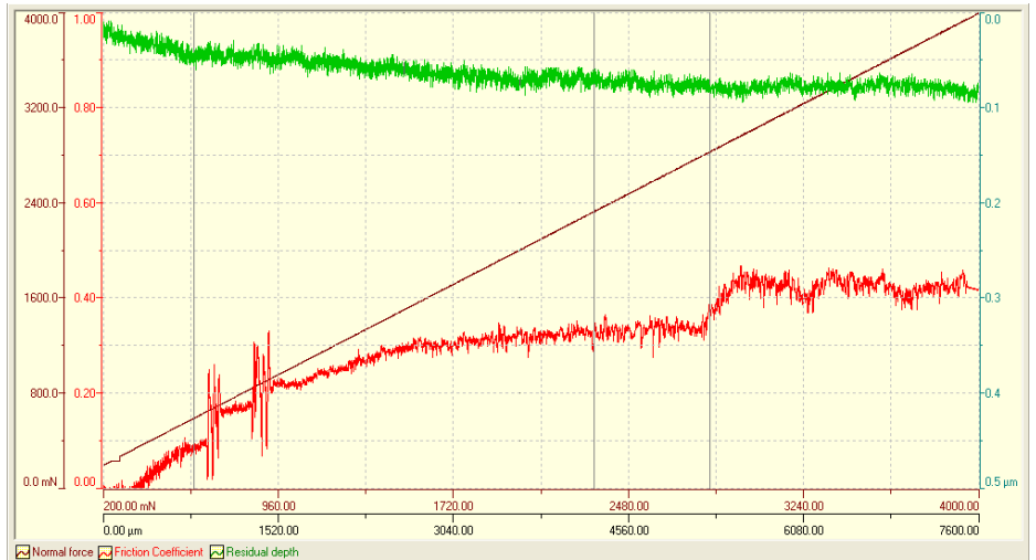
Figure 5. Scratch test results of a DLC coating. Critical loads of failure are indicated by the vertical lines.
